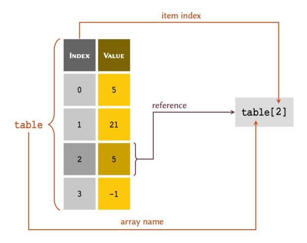
As illustrated in this figure; in order to retrieve a member of an array through its index, we write the name of the variable immediately followed by the index value inside a pair of square brackets — e.g. table[2]. Note, you may have noticed our interchangeable use of the terms 'list' and 'array'. That is because a list, in Python, can be considered as a type of dynamic array (they can increase or decrease in size, as required).
