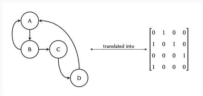
where each row in the matrix represents a node of origin in the graph, and each column a node of destination:
